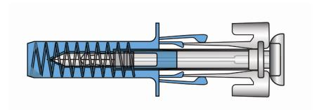
After the medicine has been injected the syringe guard will be activated to cover the needle. This is intended to protect against accidental needle stick injuries.
